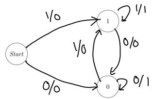
3.3 Write an FSM that will output a 1 if it recognizes the regex pattern {10+1}
